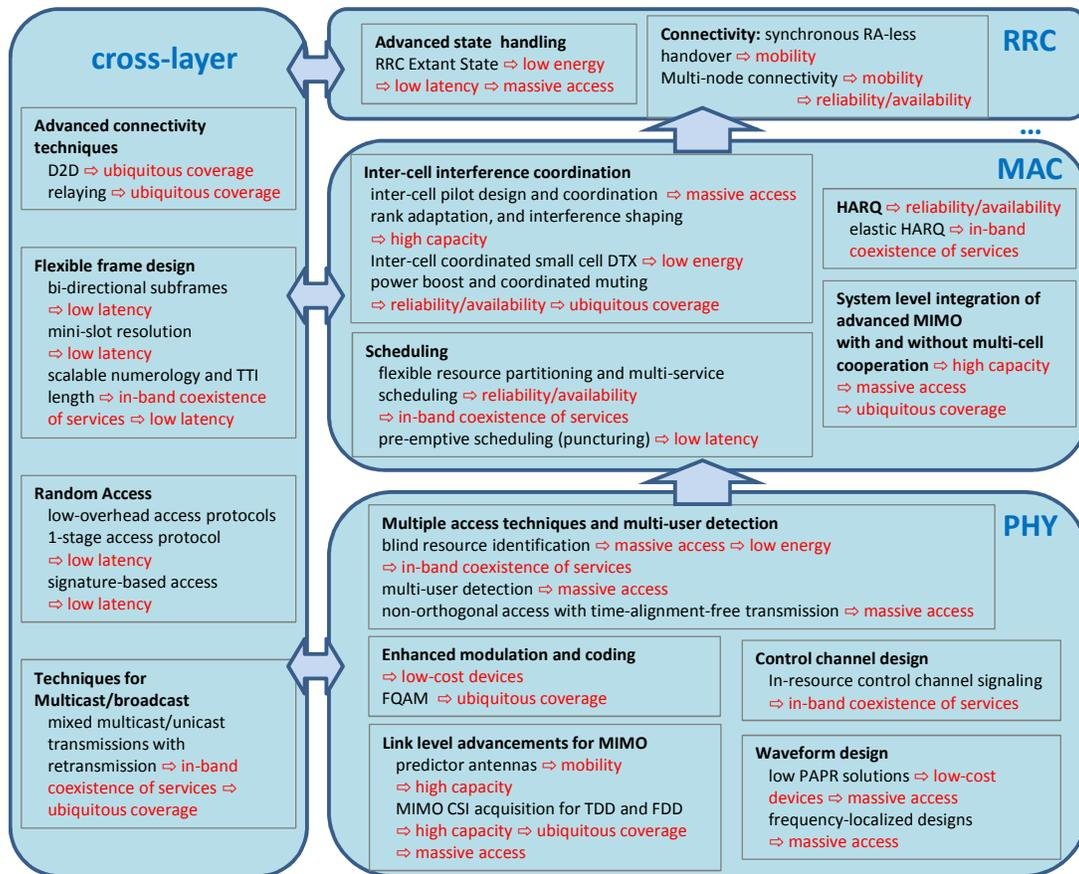
Figure 2-1: Illustration of the FANTASTIC-5G air interface with integrated technical solutions from WP3 and WP4.
